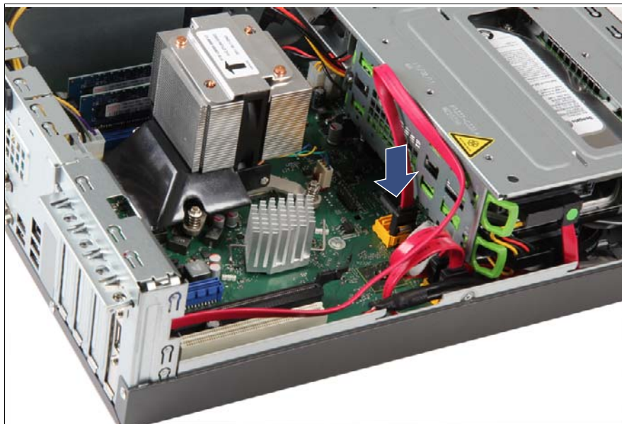
Figure 104: Connecting the eSATA cable
